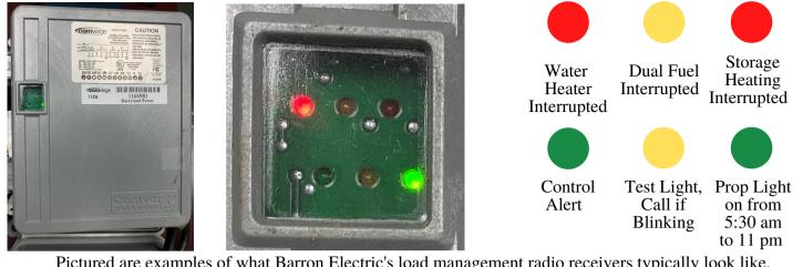
Pictured are examples of what Barron Electric's load management radio receivers typically look like. The receiver has a small window with lights that indicate the signals the radio is receiving. The graphic on the far right specifies what each light means.
