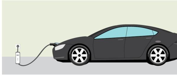
Requires access to a 120-volt outlet in an area where you can recharge the car in 22 hours (or have a qualified electrician install one in a convenient location).
