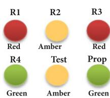
Red light on (R1): Water Heater Interrupted Amber light on (R2): Dual Fuel - Electric Heat Interrupted Red light on (R3): Electric Storage Heating Interrupted Green light on (R4): Control Alert Green light (Prop) Receiver is operating properly Prop light is on 5:30 a.m. to 11 p.m. *If you are out of hot water, please check your circuit breaker,*
