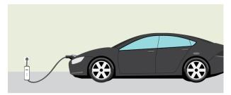
Requires access to a 120-volt outlet in an area where you can recharge the car in 22 hours (or have a qualified electrician install one in a convenient location).
