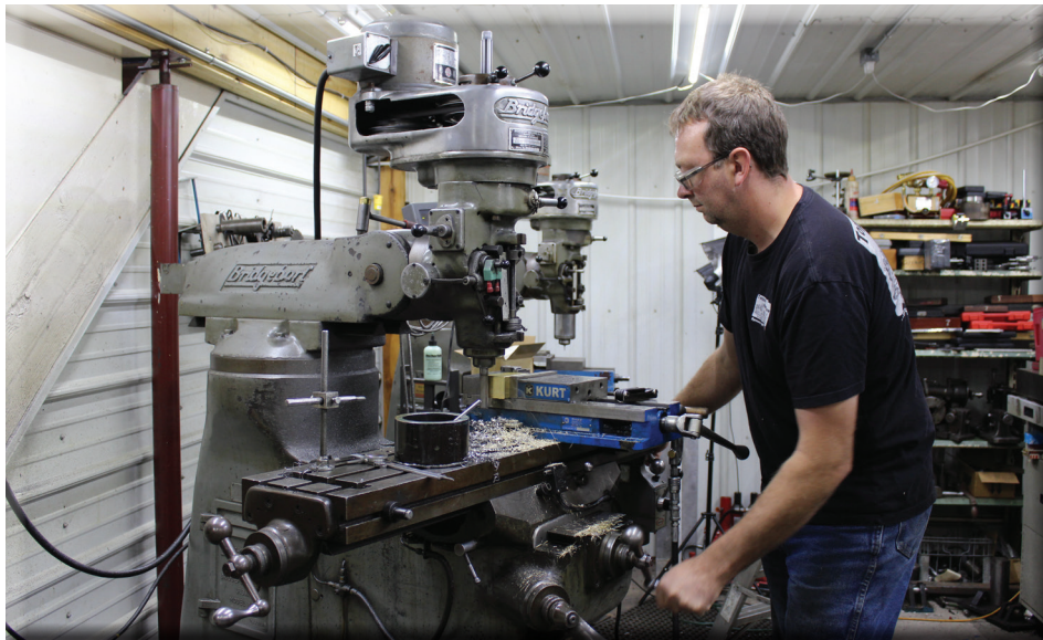
Josh Topper, Owner of Topper Machine, uses the Milling Machine to remove material from the surface of a workpiece.
