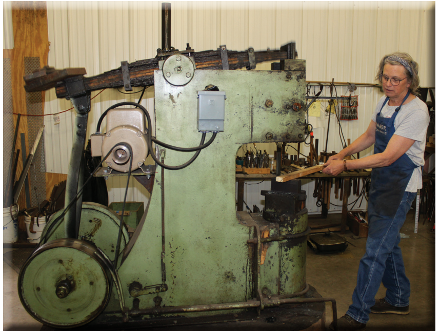
Joyce Halvorson demonstrated the antique leaf spring power hammer machine, which is used to pound heated metal into shapes.
